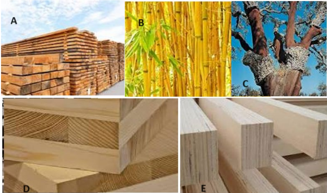
Fig. 2. Forest Material used in engineering: A, Timber; B, Bamboo; C, Cork; D, Cross Laminated Lumber, and E, Laminated Veneer Lumber
