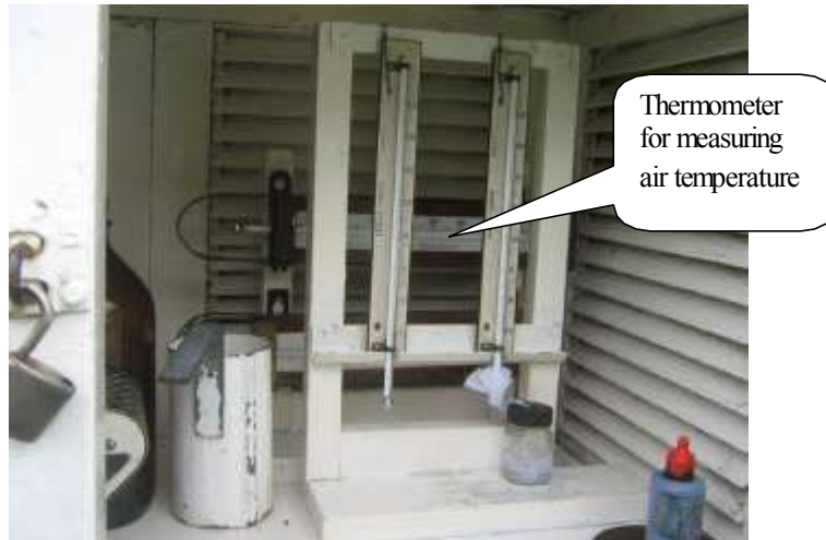
Fig. 1: The thermometer unit at Chichiri, weather station
